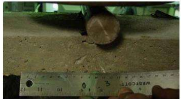
After the loading: the crack almost disappears.
