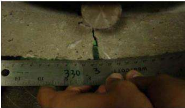
During the loading: the crack can be obviously seen.
