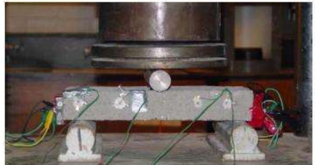
The three-point bending test of the specimen.
